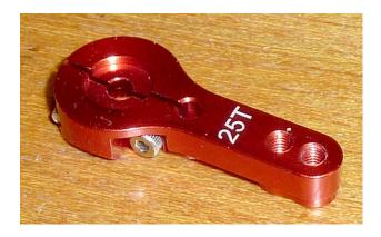
I do find the choice of an odd number of splines rather illogical. It means that, in its neutral position, you can only fit the servo arm at right-angles to the servo body on one side of the servo. On the other side it will always be slightly out as you have to move it round to find a groove. The splines are 360/25 degrees apart. So you have to move half this, or about 7°, one way or the other.
